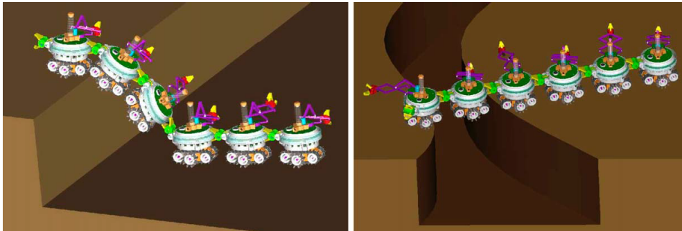
Figure 2.6: Two swarm-bots, each consisting of six s-bots, in simulation: the left one is moving down a stair, the right one is crossing over a hole. Both images are taken from [MPG + 04].
