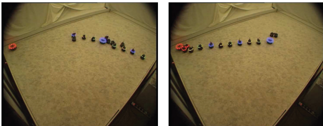
Figure 3.5: Foraging via chain forming: each robot follows a set of conditions that trigger transitions between different behaviors. In the left picture, robots have built two short chains that both do not yet reach the food item in the left corner of the area. In the right picture, one long chain to the food item could be created and two robots are already attached for transportation. Both images are taken from [NGB + 09].
